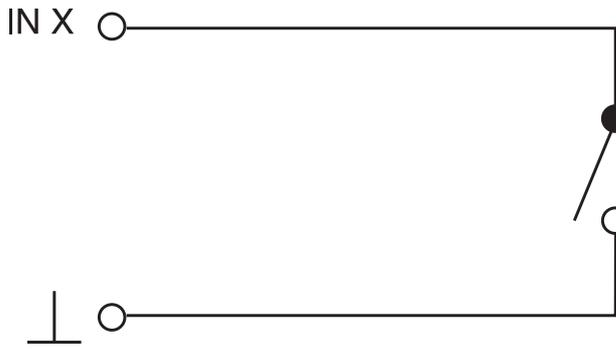
**Example wiring diagram for mode 12, 13 – monitoring device status for relay control**
