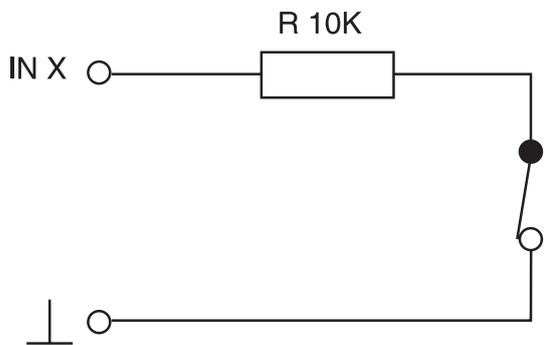
**Example wiring diagram for mode 9 – switching control input**
