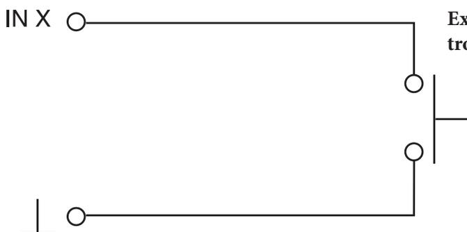
**Example wiring diagram for mode 6 - external RELAY 2 control button of in flip flop mode**
