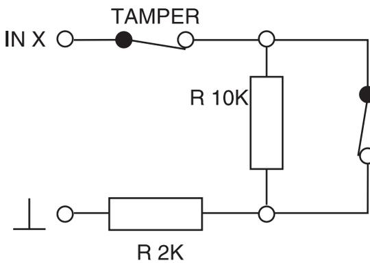
**Example wiring diagram for mode 2,3,4,5 – double balanced input**
