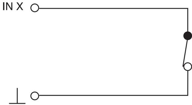
**Example wiring diagram for mode 7 – input function inhibiting output response to a ring-through**
