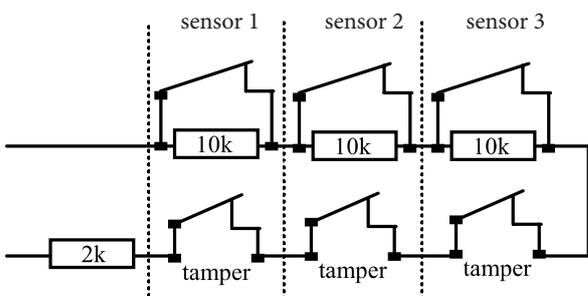
**Example wiring diagram for up to 3 sensors connected to a single loop**
