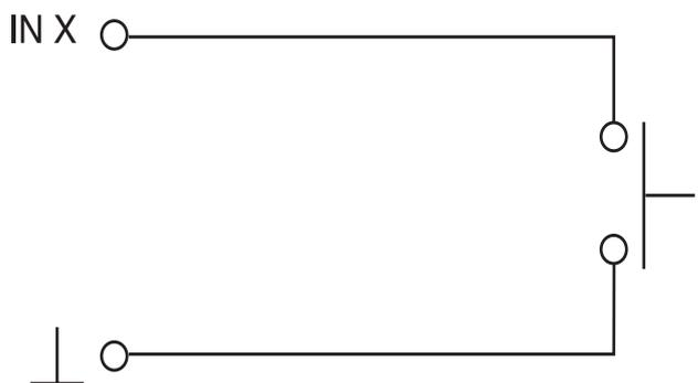
**Example wiring diagram for mode 10,11 – control button of remotely controlled relays**
