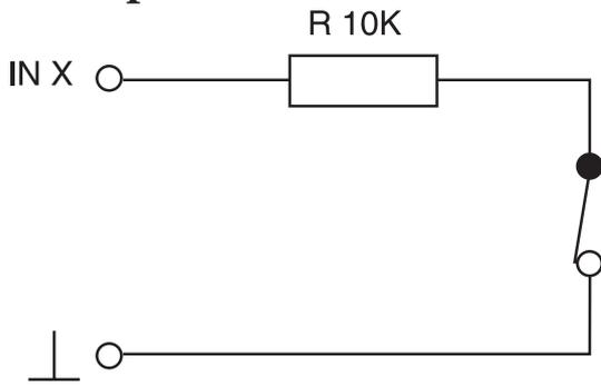
**Example wiring diagram for mode 1 – single balanced input**
